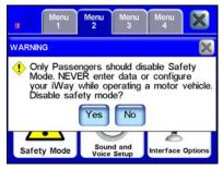
The red X on the Safety Mode button (left) indicates the feature is turned off. The disable Safety Mode Warning dialog box is shown at right.
